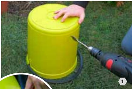
**B** Take the other two buckets and drill about 25 6mm holes in the base of each bucket. **4** Drill a few holes into the sides too. **5**
